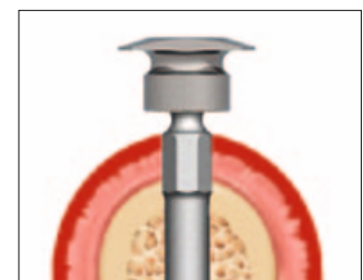
Fig. 24: The Retentions Cap Dalbo®-PLUS elliptic with Lamellae Retention Insert
